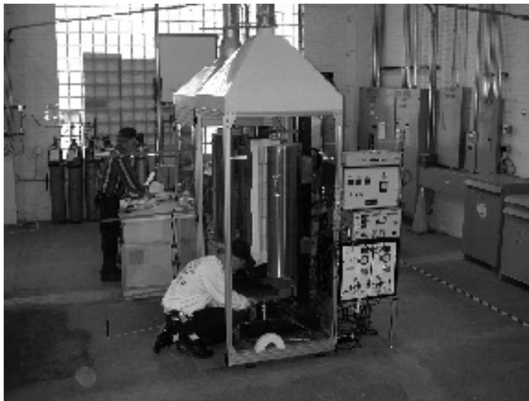
*Two PEEI technicians, Bill Evans and Jason Havash are assembling a 2<sup>nd</sup> Electrochemical Vapor Deposition system used in the Derry plant for fuel cell manufacturing.*
