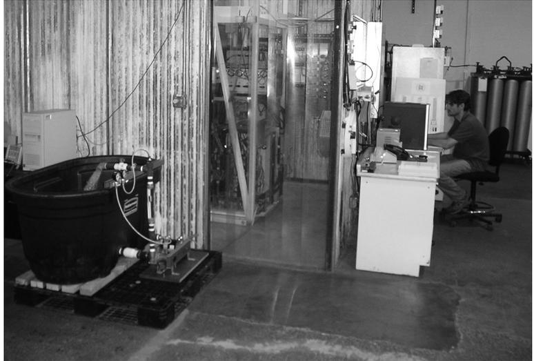
The bundle test was run at different operating conditions to provide our first operational control of an integrated system as will be required for a vehicle drive system. This demonstration maintains focus on the target application: direct (clean) replacement for diesel engines in heavy highway trucks. PEEI has manufactured and tested individual cells and is now testing a bundle which will be the standardized building blocks for fuel cell engines.
